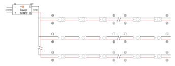
! 20 pcs - max number of modules in one chain when the power supplied from single end. ! String end voltage can't be less than 11V, do not exceed specified module string length
