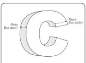
Noting metal box depth, width and face material, use layout guidelines and power supply capacity charts on page 2 to determine spacing and quantity of LEDs.
