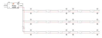
! 25 pcs - max number of modules in one chain when the power supplied from single end. ! String end voltage can't be less than 11V, do not exceed specified module string length
