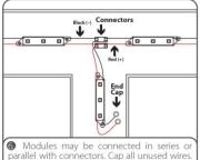
parallel with connectors. Cap all unused wires. The strand of modules should not be looped to create a closed circuit.
