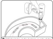
Drill the holes at the bottom or side of the letters for the wire connection to DC power supplies and grommet the hole for supply wire access.
